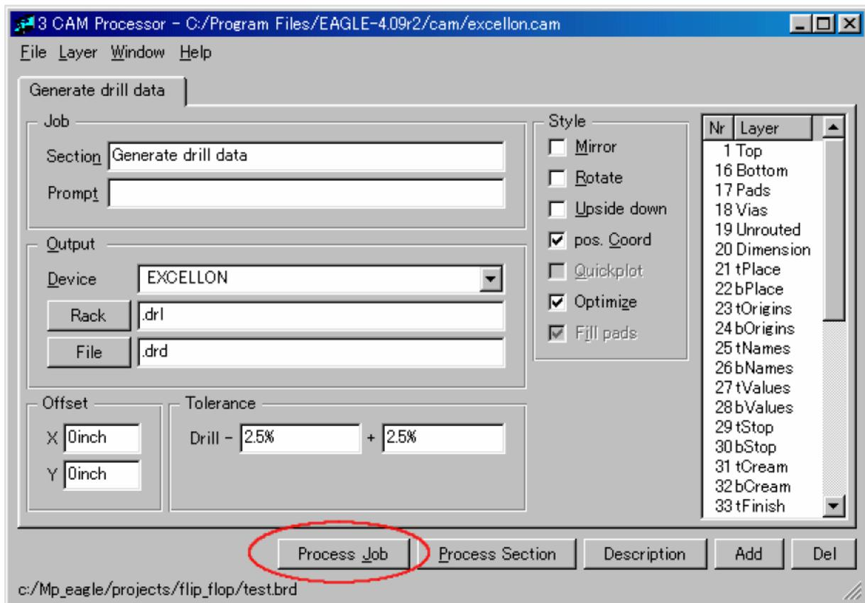
Check the items setup of Generate drill data, and push the "Process Job" button.
