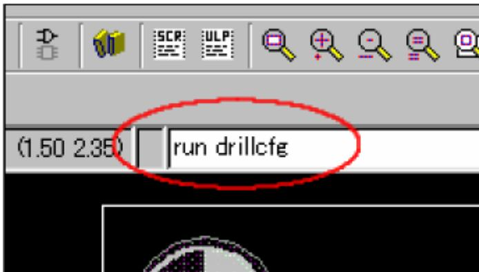
Type in "run drillcfg" to a command bar, and push an enter key.
