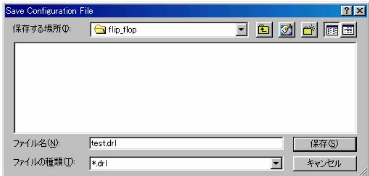
The dialog which saves a Drill Rack file (\*.drl) is displayed. You have to save this file in the same folder as a board file (\*.brd). The information written to the board file is used in CAM Processor
