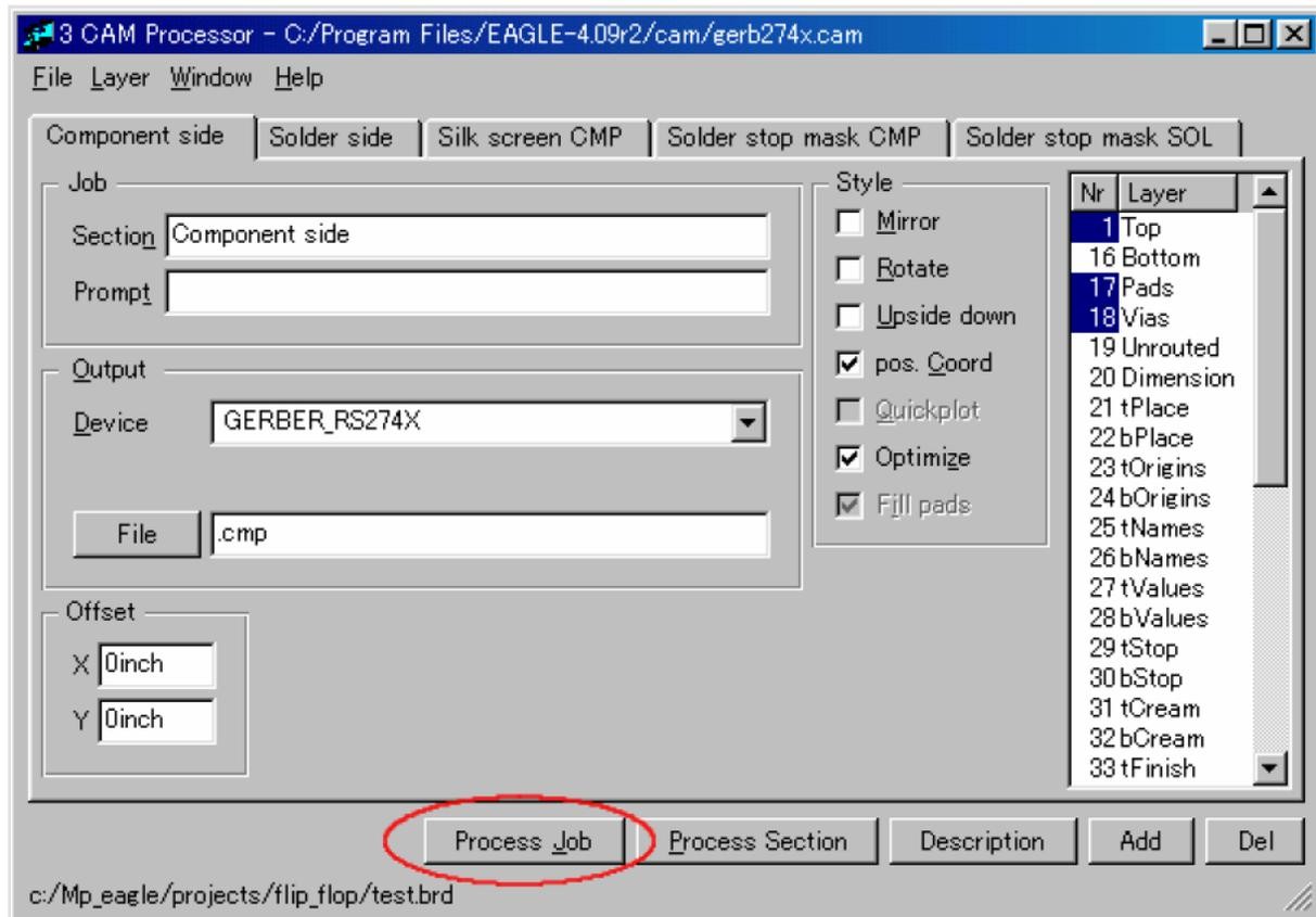
Check the items setup of Generate drill data, and push the "Process Job" button. The setting items are left default when details are not known. The Gerber files ( \*.cmp, \*.sol, \*.plc, \*.stc, \*.sts, \*.gpi ) are made by this processing.
